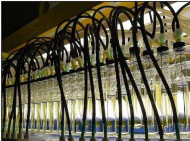
Rows of microalgae containers, removing CO 2 from the air and converting to usable products, fuels, chemicals and food.
